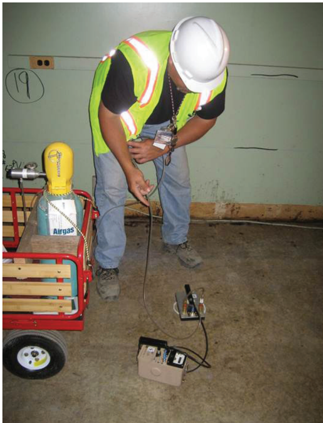
Radiological Technician takes a measurement to detect surface contamination
